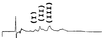
FIGURE-1(b)* : HPLC Chromatogram of fresh petrol (1% v/v in methanol) at 285 nm UV-detection.
